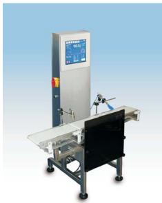
Automatic checkweighers series DWT/HL/HP are dedicated mainly for systems of Control of Packaged Goods. They are manufactured in stainless steel technology, and used in food industry.
