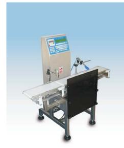
Automatic checkweighers series DWT/HL/H are dedicated mainly for systems of Control of Packaged Goods. They are designed for load with maximal capacity 7,5 kg. they are applied by food, cosmetics and chemical industry.
